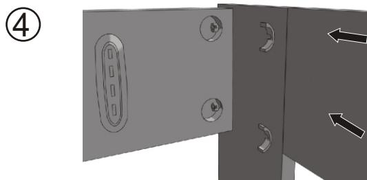
VLOŽTE KOVOVÝ SEGMENT ("MĚSÍČEK") DRÁŽKOU PŘES TĚLO ŠROUBU DO OTVORU VE VNITŘNÍ PI OŠE POSTRANICE TO SAMÉ PROVEDETE SE ŠROUB.
