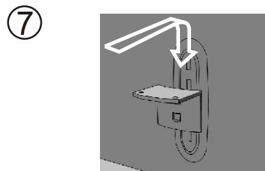
BALENÍ OBSAHUJE 6 KUSŮ NOSNÝCH PATEK VE TVARU "L", KTERÉ SE VŽDY PO 1 KUSU ZAVĚSÍ DO PŘIPRAVENÉHO KOVÁNÍ NA BOČNICÍ A ČELECH POSTELE.
